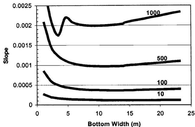
**Fig. 3.** Analytical stable channel solutions for sand-bed channels with different inflowing sediment concentrations. Solutions based on trapezoidal channel with 2:1 ( $H:V$ ) bank angles, the Brownlie (1981) depth predictor and sediment-transport equations,  $Q = 10 \text{ m}^3/\text{s}$ , and  $d_s = 0.5 \text{ mm}$ . Note that upper curve depicts shift to upper regime bedforms at smaller widths occurring at that transport capacity
