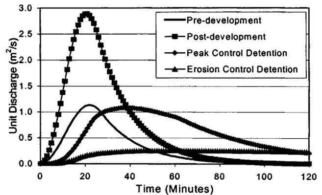
Fig. 1. Estimated Mail Creek unit discharge (2 year). Erosion control detention based on Meyer-Peter and Müller relationship using 8 mm gravel
