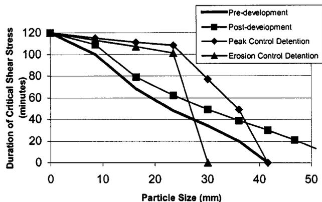
**Fig. 2.** Frequency and duration of critical shear-stress exceedence computed for four scenarios. Erosion control detention based on Meyer-Peter and Müller relationship using 8 mm gravel
